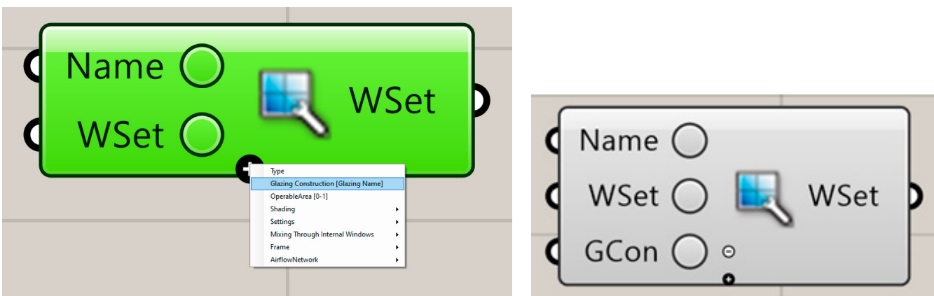
Figure 3 "CS Window settings" components, Left: Click on "+" sign and then on "Glazing Construction [Glazing Name]". Right: The input "GCon" will now appear
